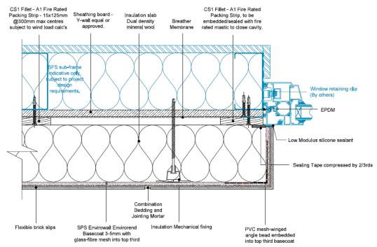
Diagram 5 - Horizontal fire barrier detail
