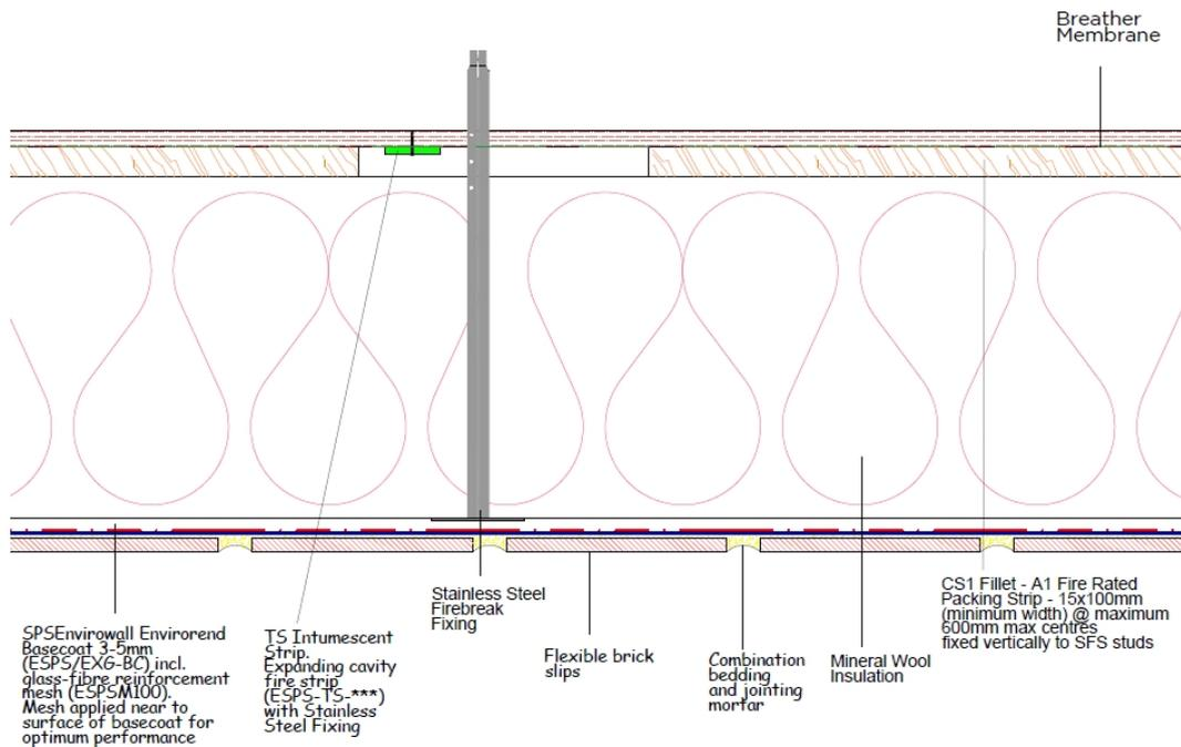
Figure 3 - Window reveal detail
