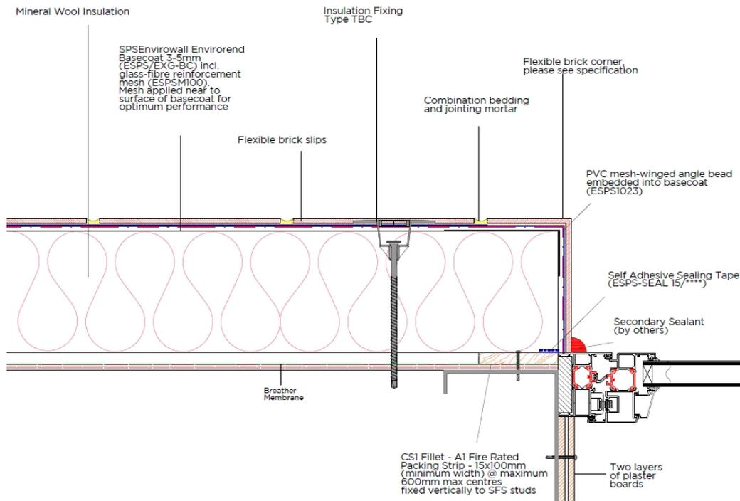
Figure 4 - Vertical firebreak detail
