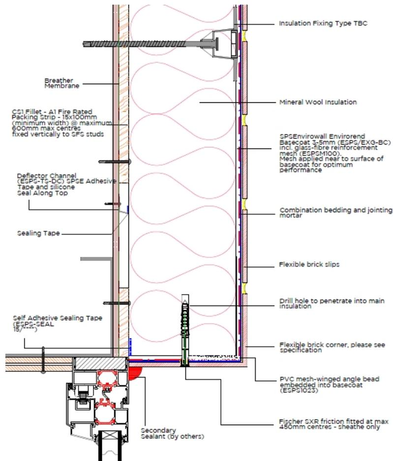
Figure 6 - Horizontal movement joint detail
