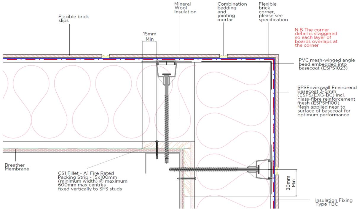
Figure 2 - Horizontal firebreak detail - plan view
