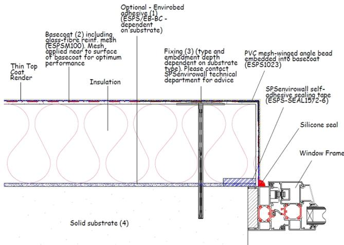
Figure 4 - Window head detail
