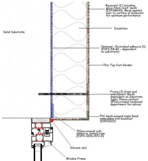
Figure 5 - Horizontal movement joint detail
