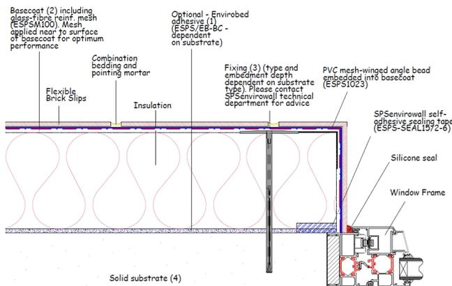
Figure 4 - Window head detail
