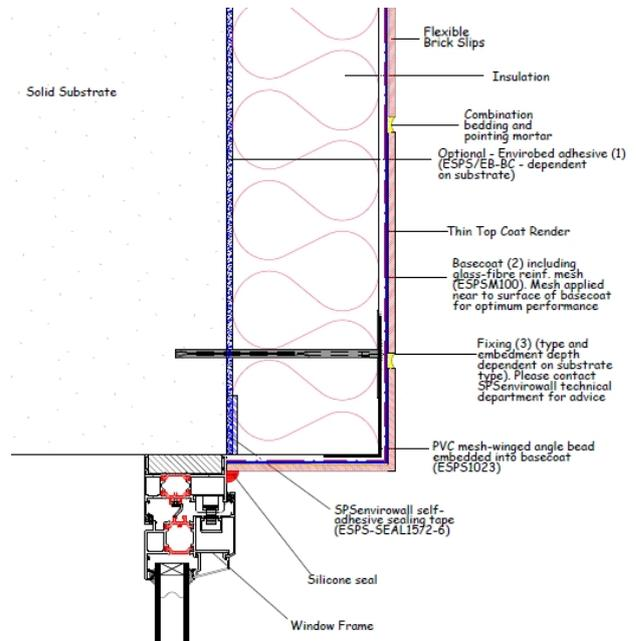
Figure 5 - Horizontal movement joint detail
