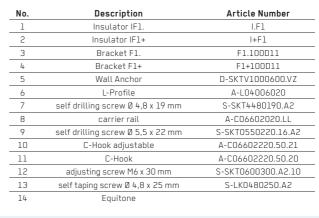
Tergo is a system for secret fixing EQUITONE panels (12mm) to the Allface System F1.40. The panels have factory drilled undercut fastener holes in the back of the panel. Hanging hooks are attached to the panel with either special rivets and spacers or undercut bolts and washers.
