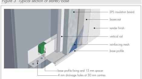
Figure 3 Typical section of starter/base
