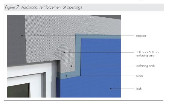
16.18 After sufficient stabilisation of the installed insulation system (normally 48 hours), during which time the insulation should be protected from exposure to extreme weather conditions to prevent degradation), the wall is ready for the application of the basecoat including reinforcement mesh.
