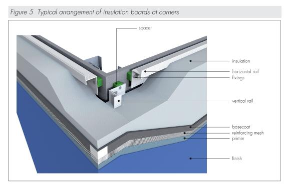
16.11 Care must be taken to ensure alignment is checked as work proceeds. The surface of the boards should be smooth without high spots or irregularities. Fire barriers must be installed where required following the designer's instructions.
