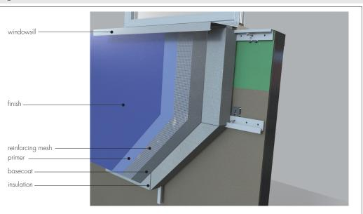
Figure 10 Insulated window reveal detail
