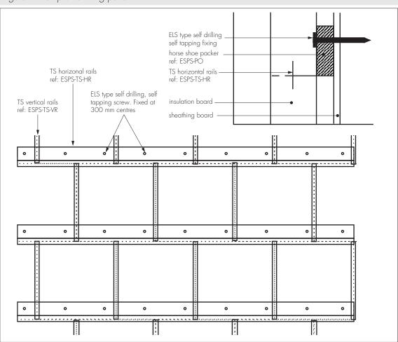
16.7 The first insulation board is positioned onto the base profile, and is used to position the first horizontal rail (see Figure 4). The fixing rail slots into the pre-cut groove in the insulation board. The level is checked and the rail is positioned away from the substrate using the 15 mm spacers. It is important that the fixing rail fits tightly and locates fully into the groove in the insulation; it should not be forced into position.
