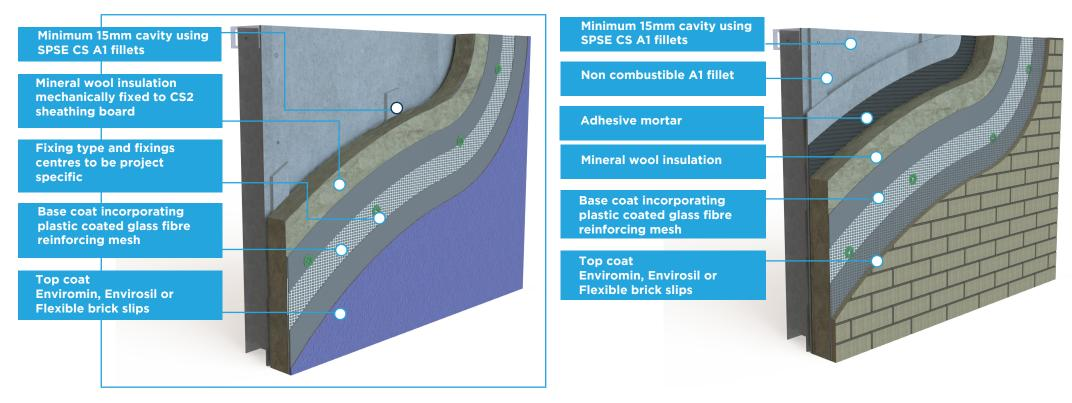
Our market-leading Cavity Systems consist of Euroclass BS EN 13501 - A1 components, which are mechanically fixed back to the inner sheathing board to create the designed cavity width with either the insulation board fitted directly to the A1 fillets (CS1 system), or a secondary A1 sheathing board and insulation (CS2 system). Our A1 EWI recladding systems are supplied with a mineral top coat finish.
