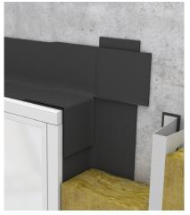
EPDM for flashing is UV resistant and is sealed around openings with EPDM adhesive.
