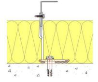
The insulation will have to be cut to allow the leg of the support profile be mounted in the bracket. But this will not affect the fixing of the profile to the bracket.
