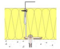
Because the fixing of the support profiles with the bracket lies in the insulation, this should be introduced only after installation of the substructure.
