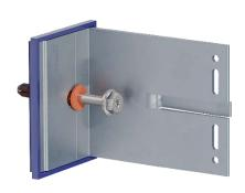
When attaching F1 brackets in masonry or concrete, make sure that the anchoring of the anchor always takes place through all existing slots (F1+). Furthermore, make sure that the plastic frame of the anchoring plug is inserted through the bracket.
