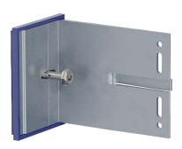
When anchoring F1 consoles on steel or wooden surfaces, make sure that the number of anchoring screws equals the number of fixing holes per bracket. The anchoring must be done in all 6.5mm slots of the console.
