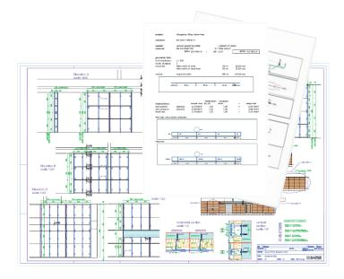
The project calculations based on the Project-Info you submit will determine the layout of the F1. and/or F1+ brackets. F1. & F1+ brackets achieve a 35 - 255mm standoff as standard, other sizes are possible and made bespoke. Other sizes can be ordered after consultation as F10 console.
