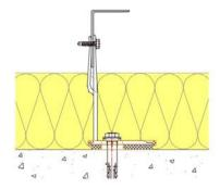
The insulation does not interfere with the profiles or brackets.
