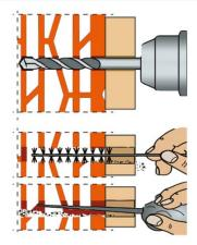
When anchoring F1 brackets to masonry or concrete, a dowel extension test is recommended to check the load bearing capacity of the masonry. All holes must be thoroughly cleaned and free of dust / dirt before using the anchoring dowels.
