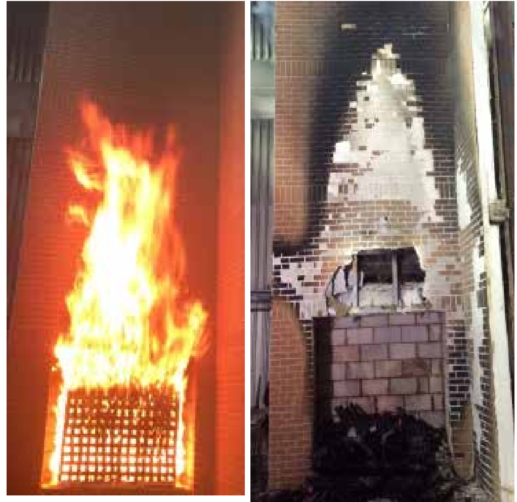
Benx Ltd EWI systems being successfully tested to BS 8414
