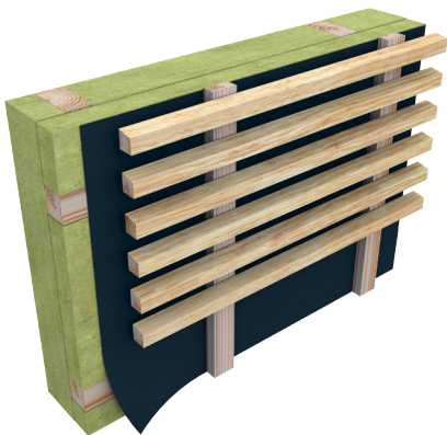
Open facade cladding.
