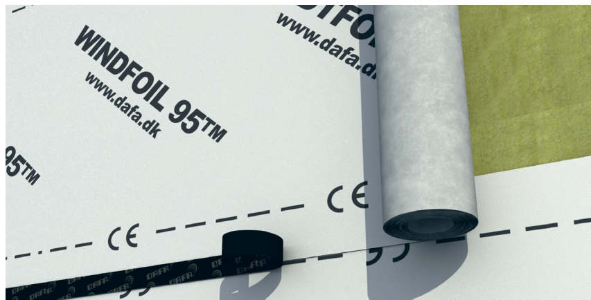
DAFA WindFoil 95 is installed as a wind barrier with a minimum overlap of 150 mm and free joints are taped using DAFA UV tape.
