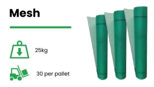
Supplied in 50m<sup>2</sup> rolls (50m long x Im wide) Benx glass fibre reinforcement mesh is used to add extra strength and impact resistance to basecoats, both in a render only context and when applied as part of an external wall insulation system. The reinforcement mesh should be applied as near to the outer surface of the basecoat as possible to provide the most effective protection.
